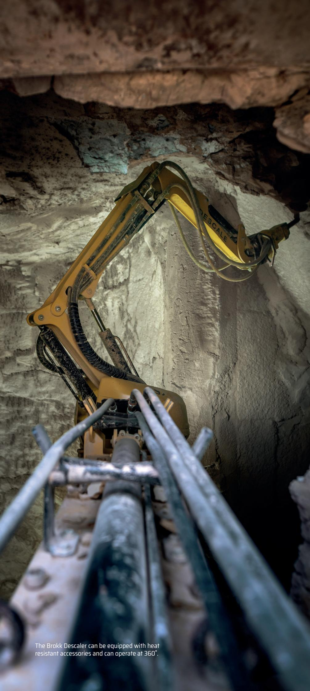
in the kiln. Only a single operator is needed working at a safe distance, and the robot is able to descale much faster than it would normally take an entire team. In an industry in which one hour of downtime implies lost production, the investment in a Brokk Descaler is very quickly paid back.
