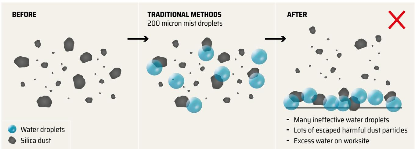
Silica particles range from 0.1 to 1,000 microns while traditional methods produce water droplets that are 200 to 1,000 microns in size.
