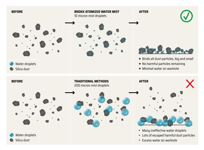
Silica particles range from 0.1 to 1,000 microns while traditional methods produce water droplets that are 200 to 1,000 microns in size.
