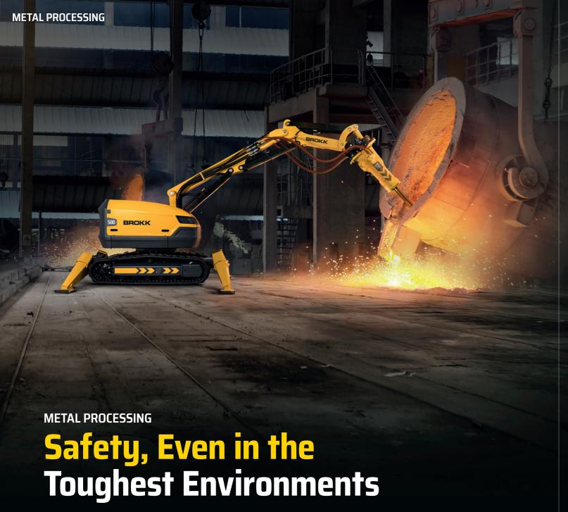
Wherever there are refractory linings or slag, Brokk remotecontrolled demolition robots will always find work. Thanks to their versatility, Brokk robots can be used in numerous applications in the metal processing industry. Their main task, however, is always the same—to minimize plant shut down time in a safe and efficient manner.
